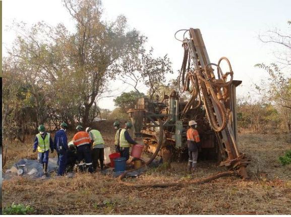
RAB Drilling at Miyabi
