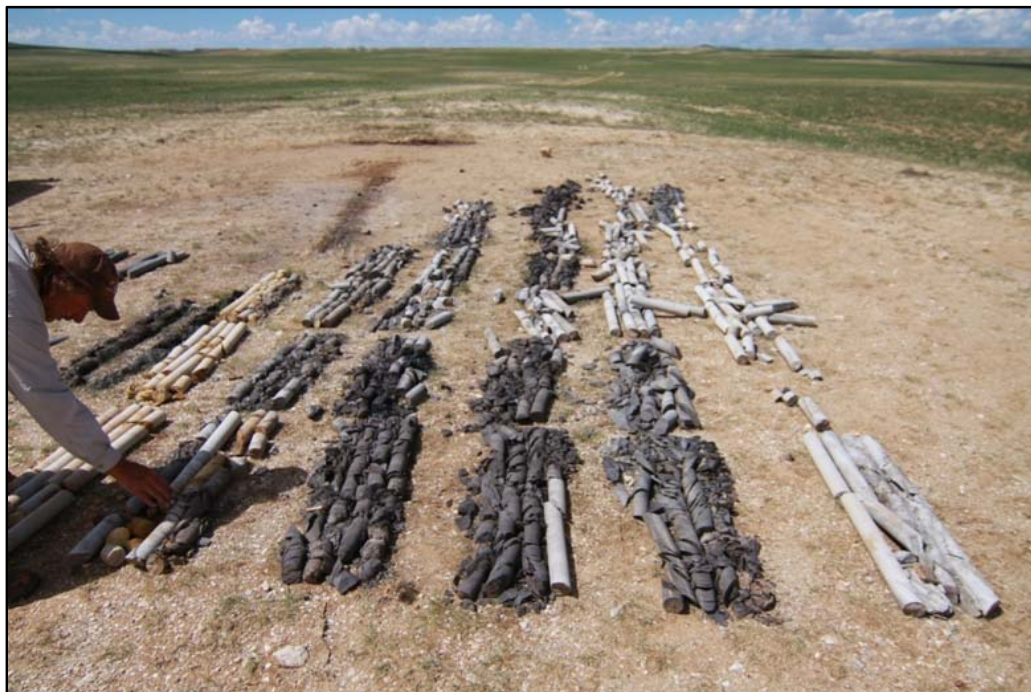
Figure 2-9: Drill Core Exposed at Wellsite BTE-002
