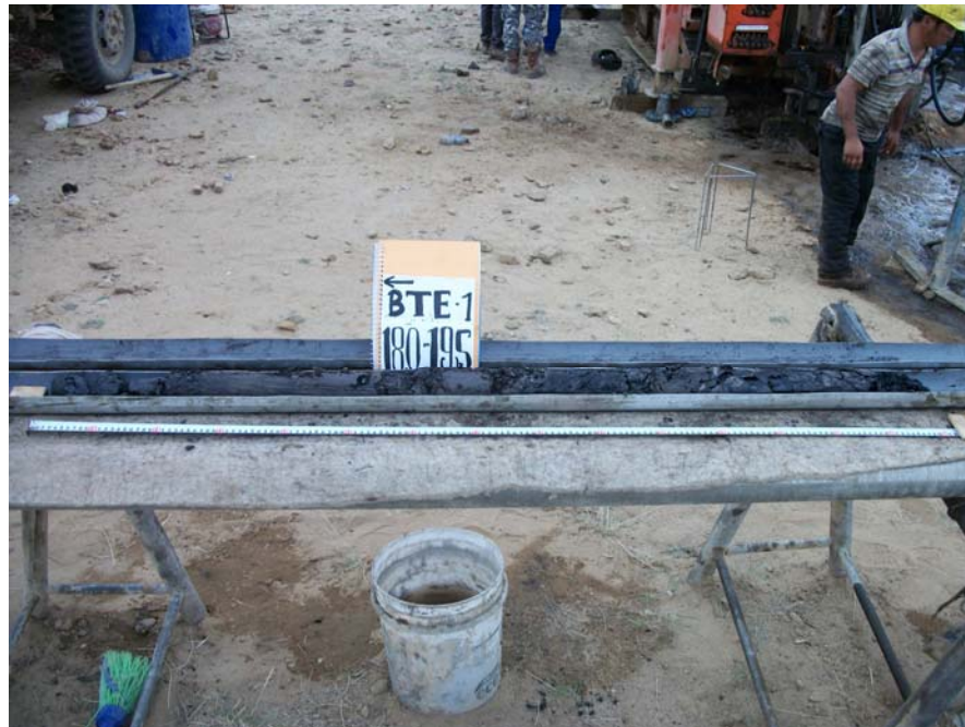
Ovorhangay Province: Drill Core from BTE-1 from 18.0m to 19.5m
