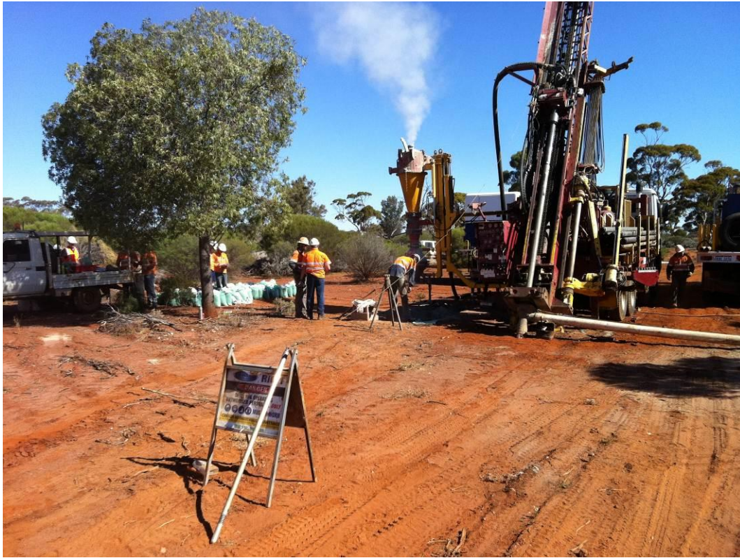
Figure 2 RC drilling at the Brilliant deposit
