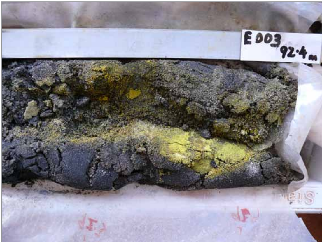
Sonic core from E003 showing yellow uranium minerals in coarse-grained sand
