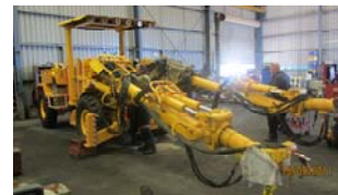
Jumbo twin boom drill rig Delivery November 2011
