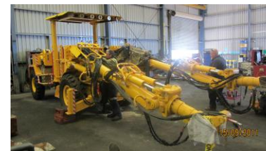
Jumbo twin boom drill rig
