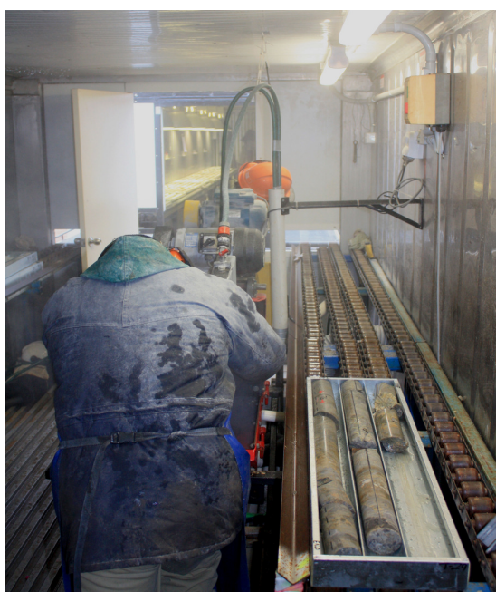
Photograph 5. Cutting drill core with a brick saw, strong suction fans remove mist and fine rock particles from the 6m converted sea container and roller tables ensure no lifting during the process of cutting 1000's of metres of core.
