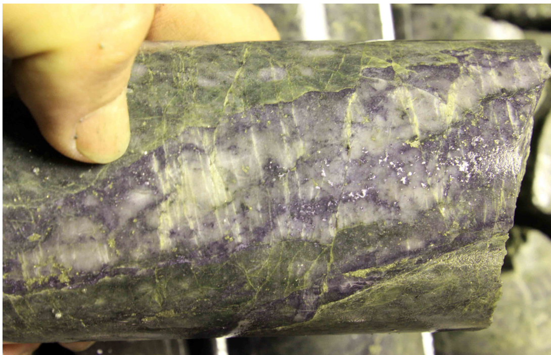
Photograph 3 DUNDD008. Example of strong visible coarse molybdenum mineralisation in quartz stock work veining - which is typical of the intersection between 340 and 387metres.
