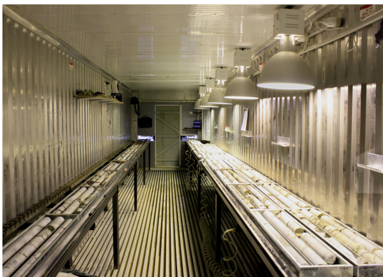
Photograph 4. Logging drill core within a 12m long converted insulated sea container, roller tables ensure no lifting of core trays throughout the logging, cutting and sampling process.
