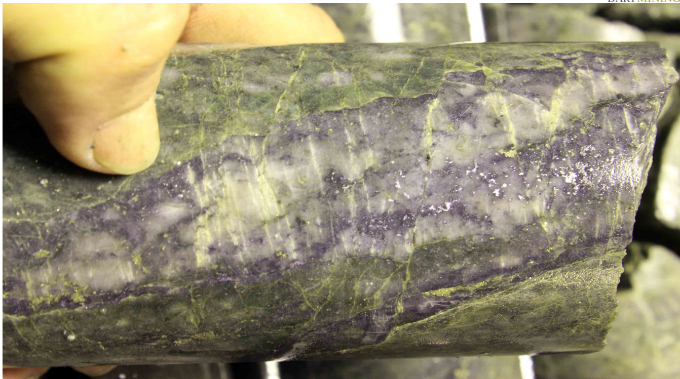
Photograph 3 DUNDD008. Example of strong coarse molybdenite mineralisation in quartz stock work veining – (2m @ 0.3% Mo and 29.1 g/t Ag – 368 -370m)
