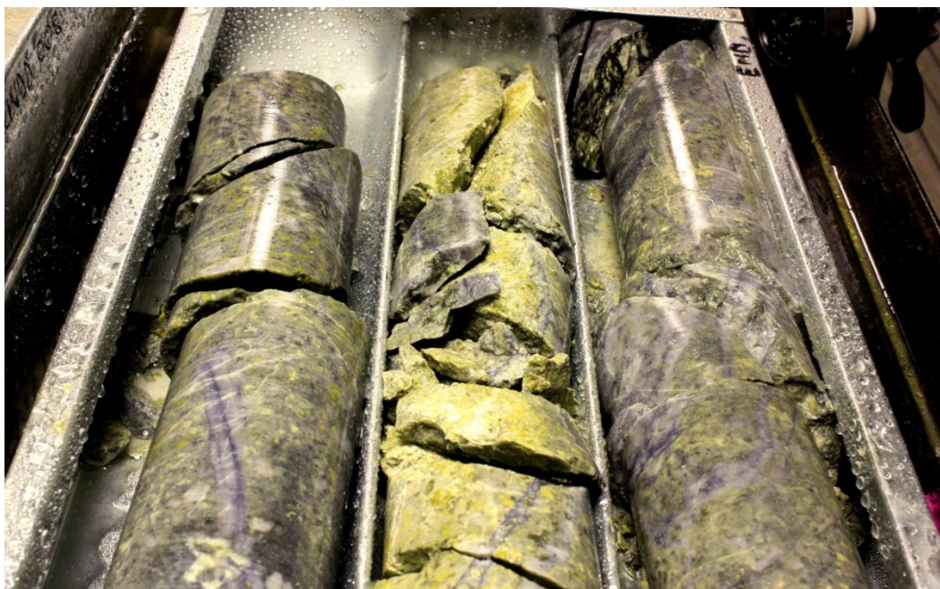
Photograph 1 DUNDD008. Average Mo grade of 0.08% over a 40 metre intersection (348 – 387.9m). Visible molybdenum mineralisation (blue veins) in dense quartz stock work veins which is typical of the high grade Mo intersection.
