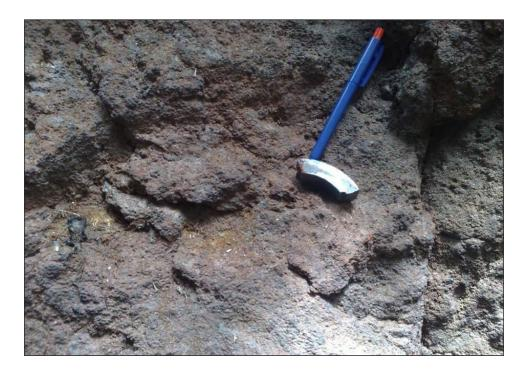
Figure 6: Oolitic Ironstone in Bulk Sample Trench – EL8886.
