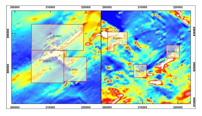
Figure 20: TMI Images Showing High Magnetic Response Associated with Magnetite Quartz-feldspathic Gneiss within some of the Portions of Basement Tenements.
