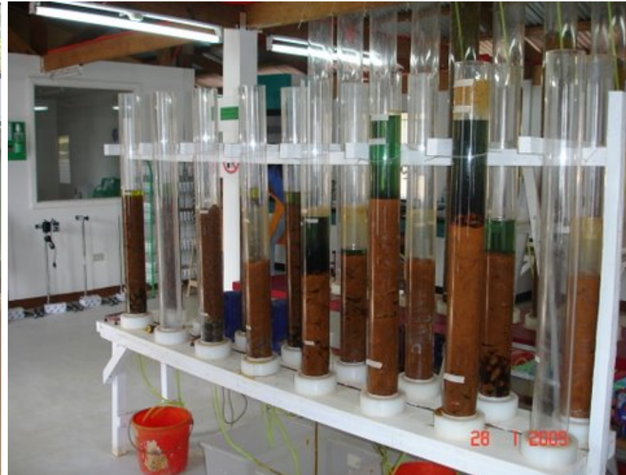
1m Percolation Columns
