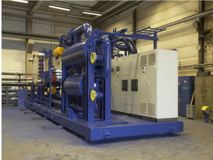
Enerji's Opcon Powerbox near completion
