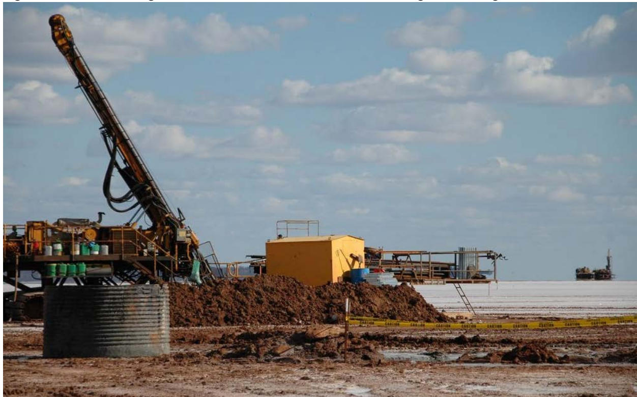
Figure 7: Diamond drill rig on lake bed at Treasure Island with aircore rig in the background.
