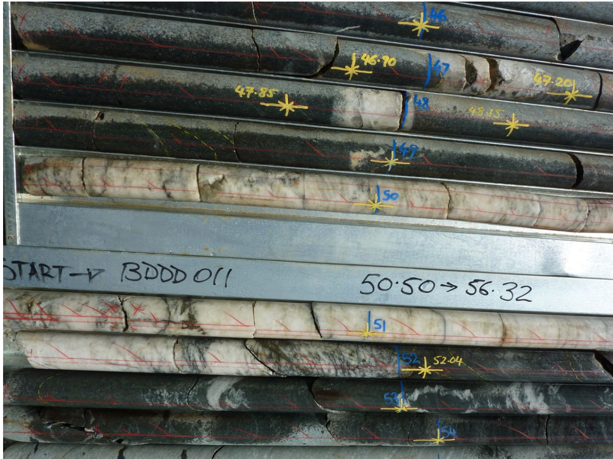
Figure 4: Drill core from BDDD011 showing a mineralised quartz vein, 2.5m @ 10.82g/t (containing sulphides & fine gold).
