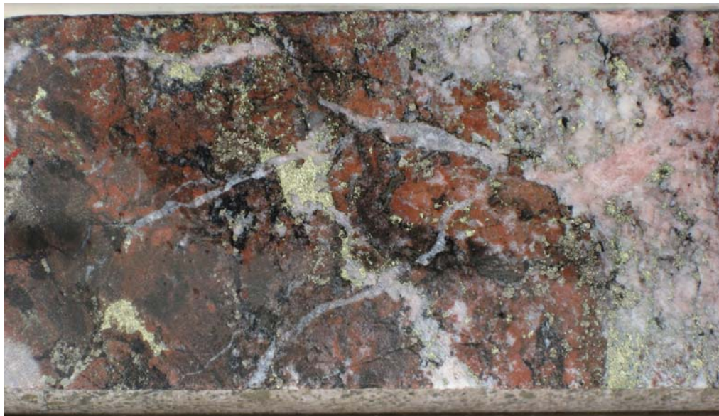
Photograph; Milo breccia with chalcopyrite mineralisation (half NQ2 core height approx. 50mm)
