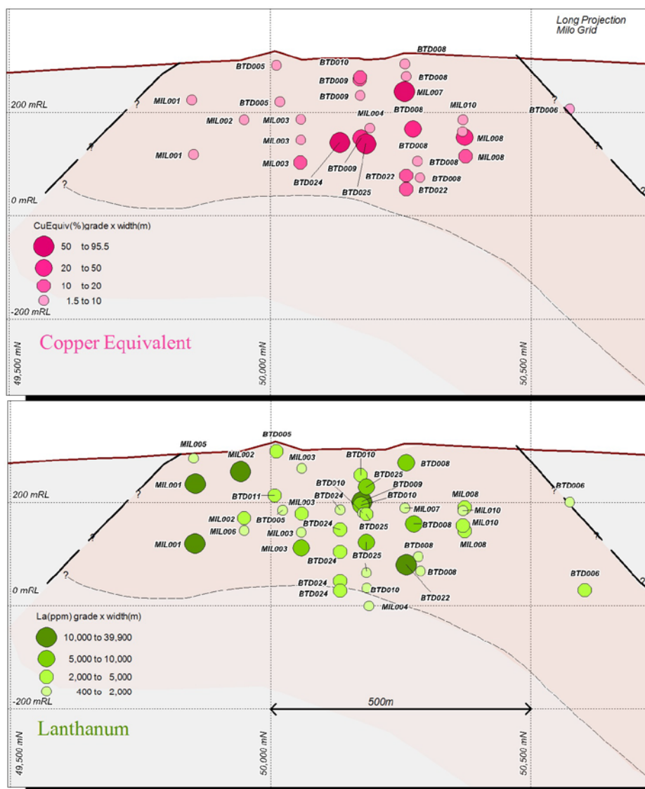
Figure; Milo Longitudinal Projection showing distribution of drillhole intersections for copper equivalent metal suite (top) and Lanthanum (bottom). Figure shows estimated true width times grade.
