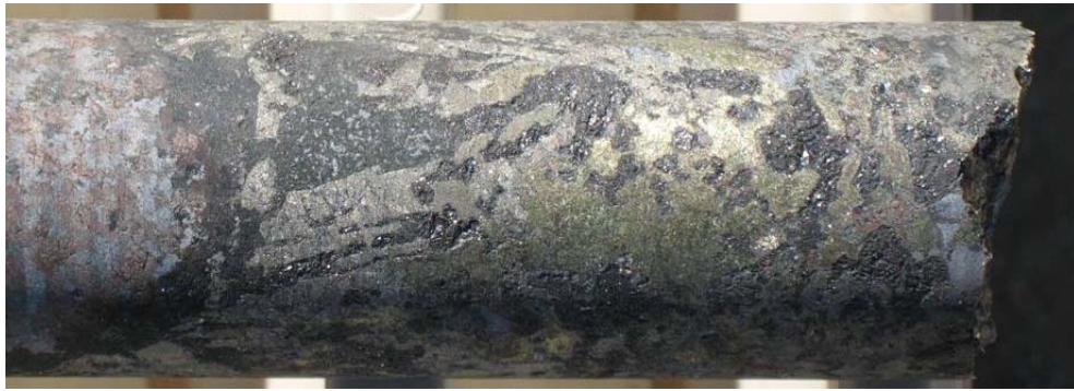
Photograph; chalcopyrite-pyrite-magnetite mineralisation in granite breccia.(NQ diamond drill core).
