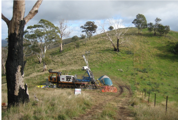
Photograph; Diamond drilling in progress on hole MGDD08 at the Monkey Gully Prospect.
