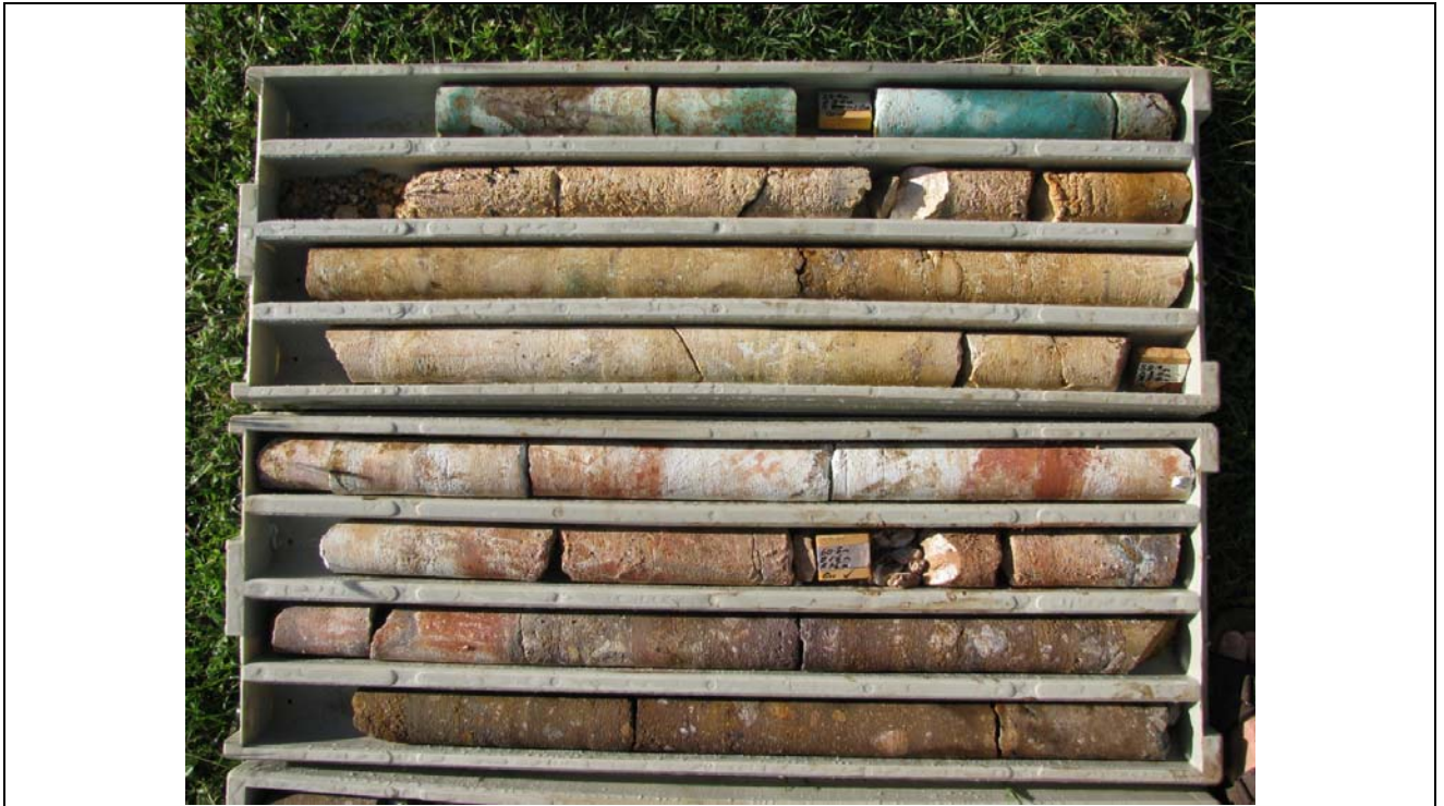
Figure Three MDD006 – Core recovered in the target breccia from 50 metres and continues at depth to 78 metres. Yellow brown rock in bottom metres is supergene Chalcocite (copper sulphide) breccia from 60.5 metres confirms the extension at depth of the Mount Dorothy sulphide breccia. The top metre is green pseudomalachite in breccia. The brown metres at the bottom of the tray average 10.5 % copper.
