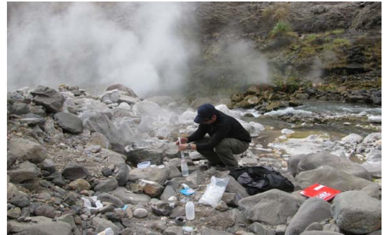
Hot springs & silica sinter at Quella Apacheta- Cation 15 geothermometry subsurface reservoir +230^{\circ}\text{C}
