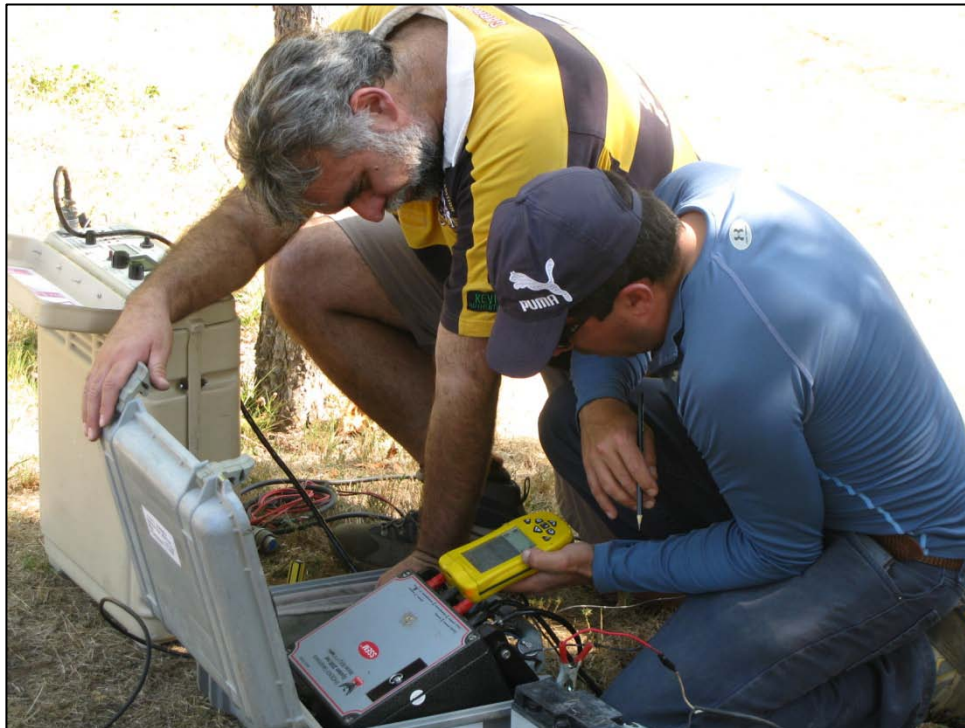
Figures 2: MT and TDEM geophysical measurements in progress at HRL's Longaví project
