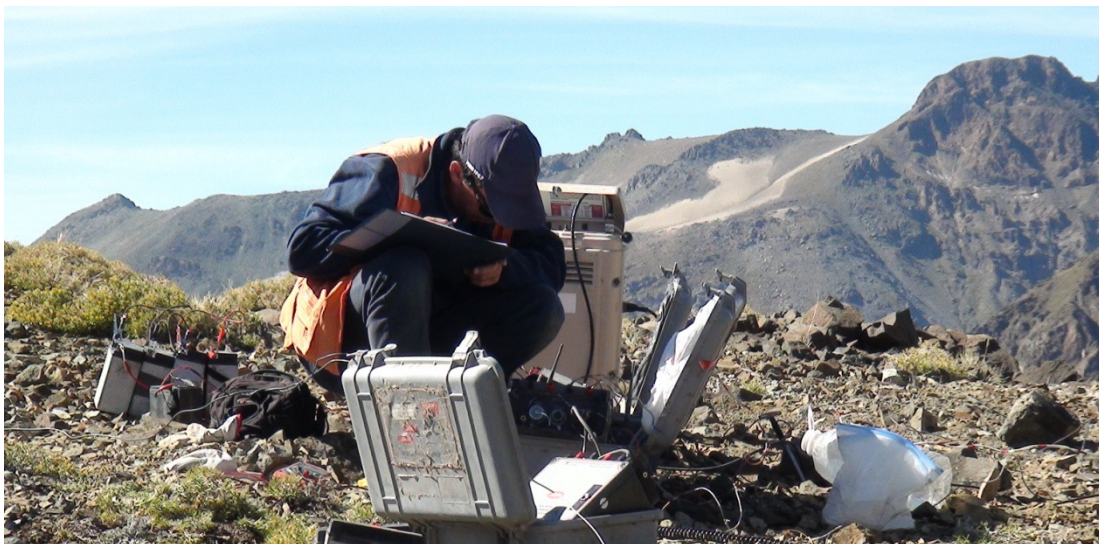
Figure 1: Field crew acquiring MT and TDEM geophysical measurements at Longavi
