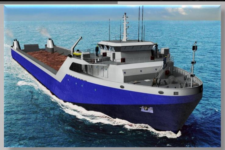
Feeder carrying 1500 dwt of bulk on 2.4m draft 3 miles to transfer vessel 12,000TPD, 4 million TPA
