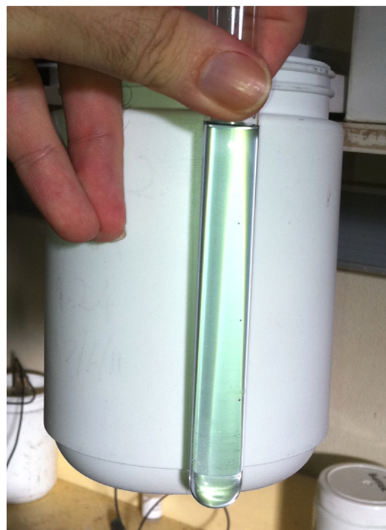
Dissolved rare earth neodymium and dysprosium elements (from industrial waste leaching & purification) in Intec Process electrolyte during recent laboratory testing.
