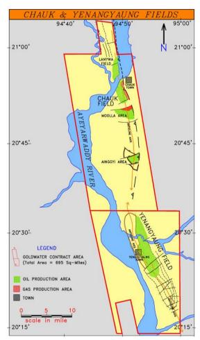
the approximately 278 kilometres of 2D seismic data acquired in 2010 over Chauk field was completed and was incorporated into the existing subsurface interpretation with the aim of delineating a potential "deep" drill site, and further field development opportunities.
