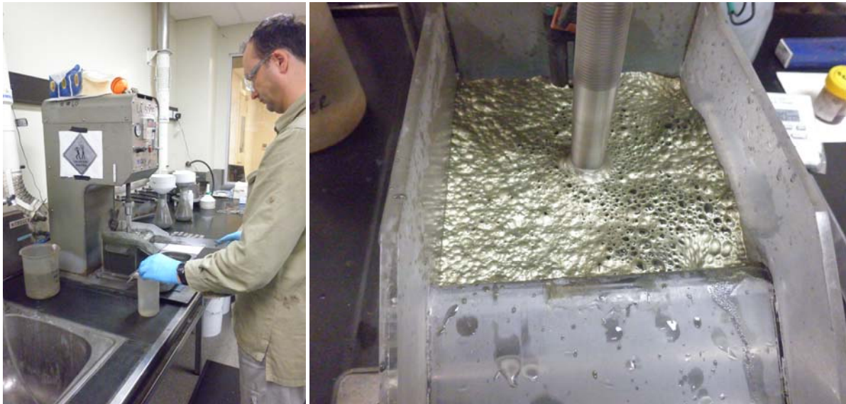
Figure 1 Jervois copper concentrate production at Ammtec laboratory
