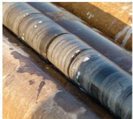
Figure 1 Carbonaceous mudstone with coaly layers emitting gas before being sealed in desorption canisters.
