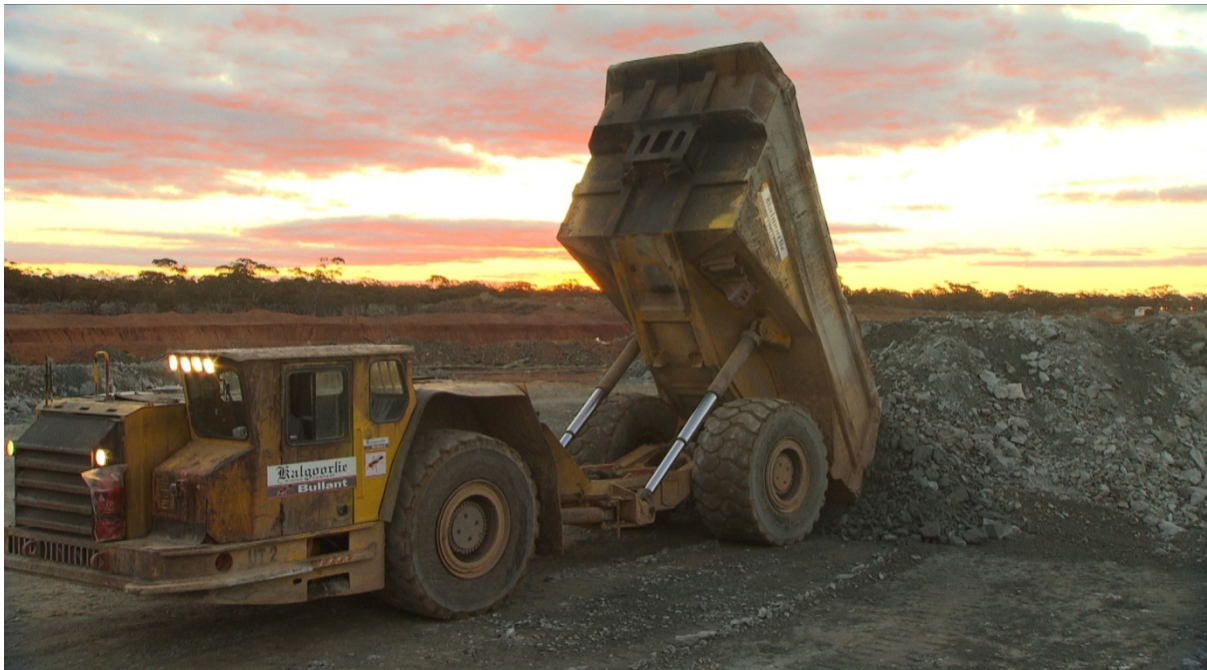
Picture 1: MT50 trucks continue to haul gold ore from the Bullant Gold Mine, grades are expected to increase with commencement of open stope mining.
