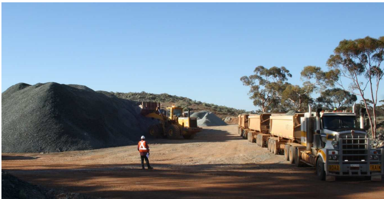
Picture 1: IES Quad-train haulage truck being loaded with ore at the Bullant Gold Mine.
