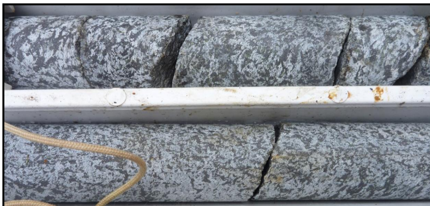
Photo 1: Magnetite Gneiss Drillcore from Drillhole DH046
