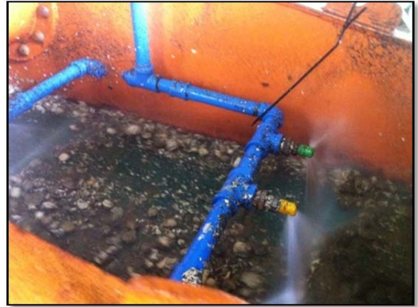
Figure 3: Screen used to remove the +1mm coarse material
