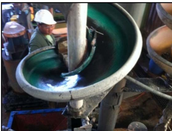
Figure 5: Spiral in operation. Beneficiated product is the dark colour (inside) and the shell fraction is the light colour (outside).
