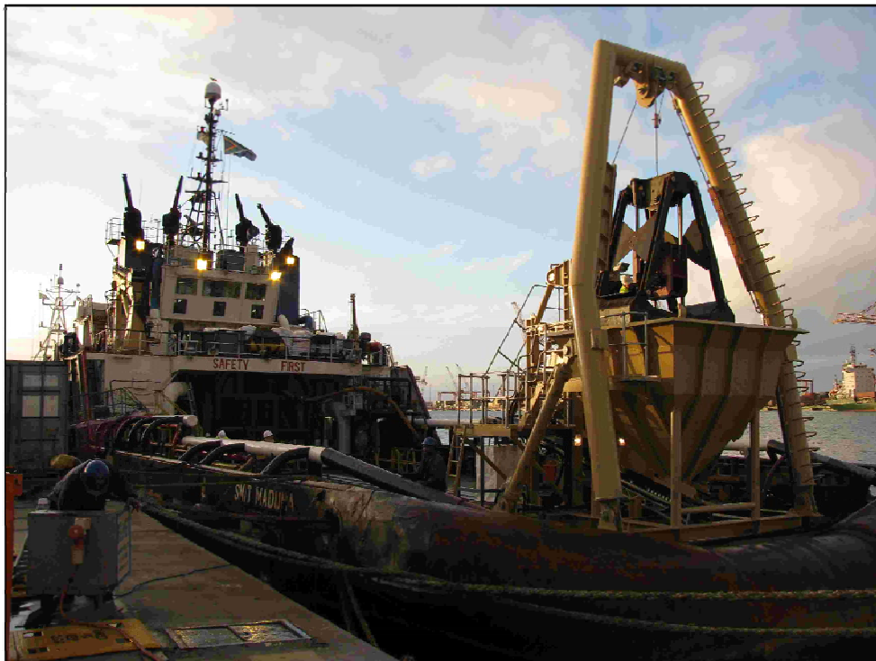
Sampling equipment installed on the MV Smit Mandura
