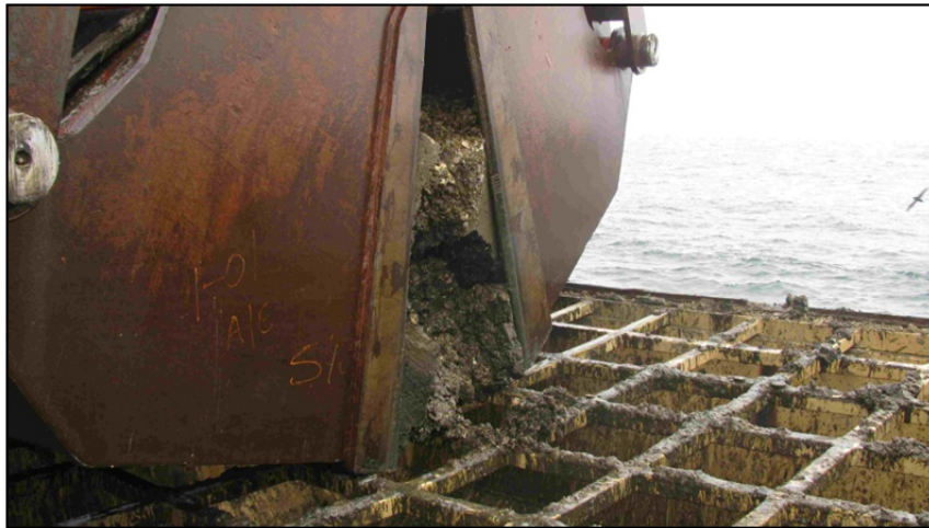
Figure 2: Unloading a 2t Sample
