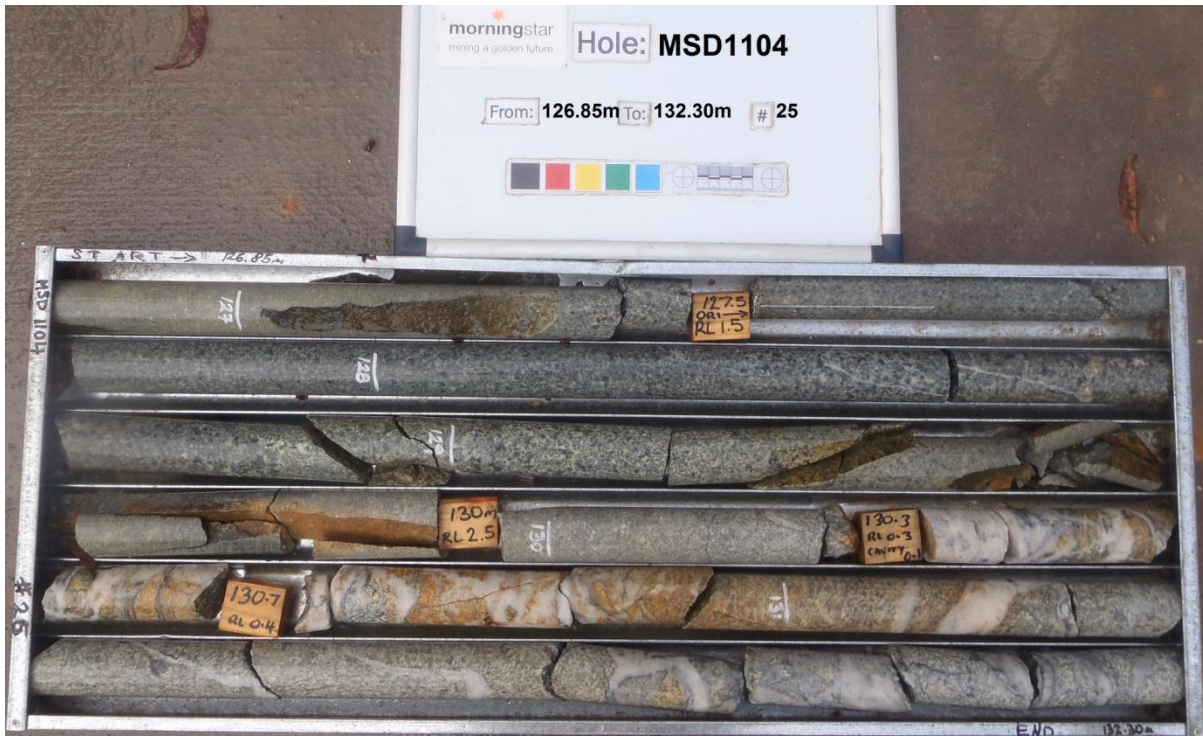
Figure 2: MSD1104 Showing Intense Alteration & Quartz Veining (incl 5.19 g/t Au @ 130m).
