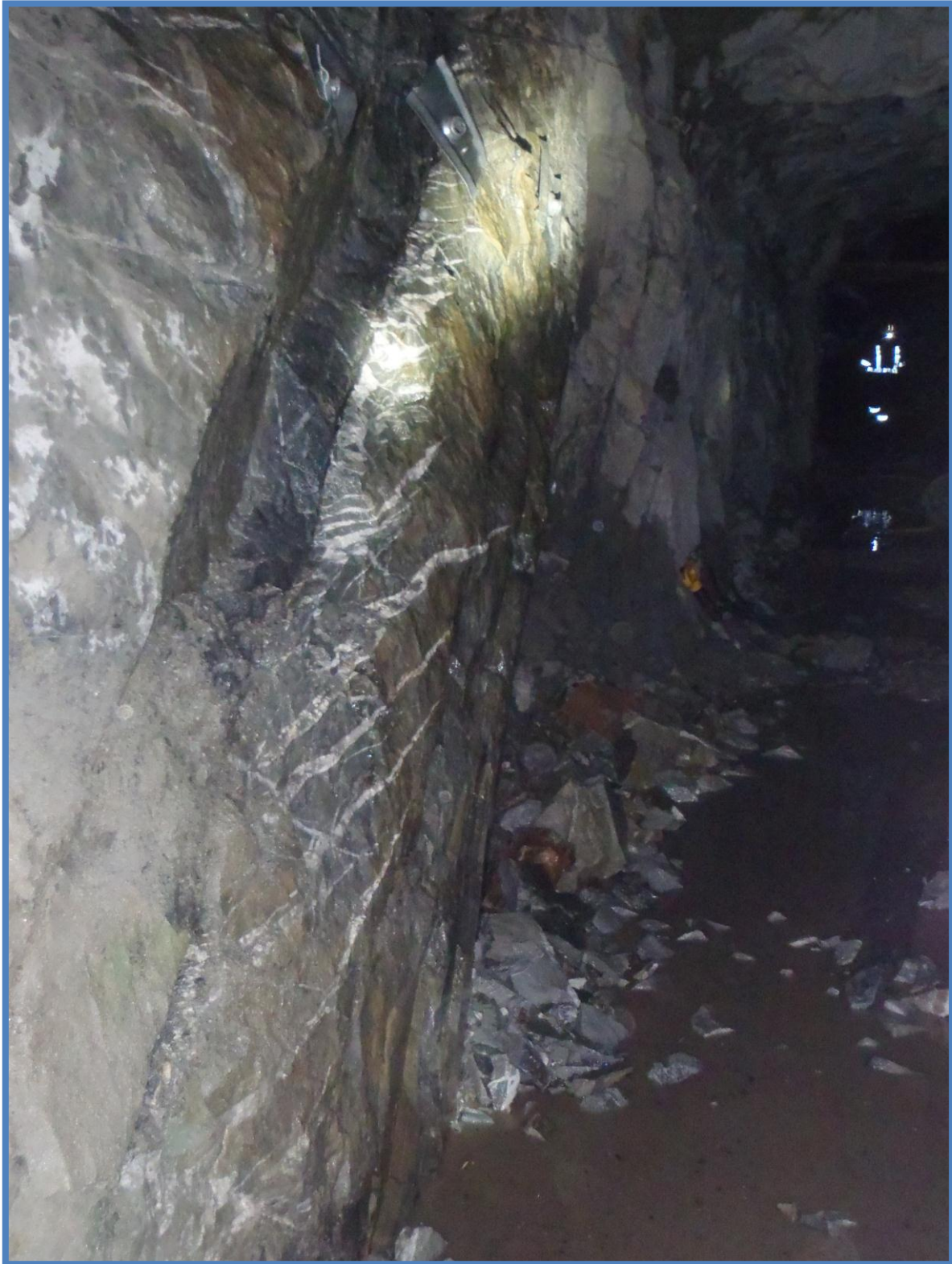
Fig 3: Location of the 851 g/t Au grab sample (note quartz veining in wall)
