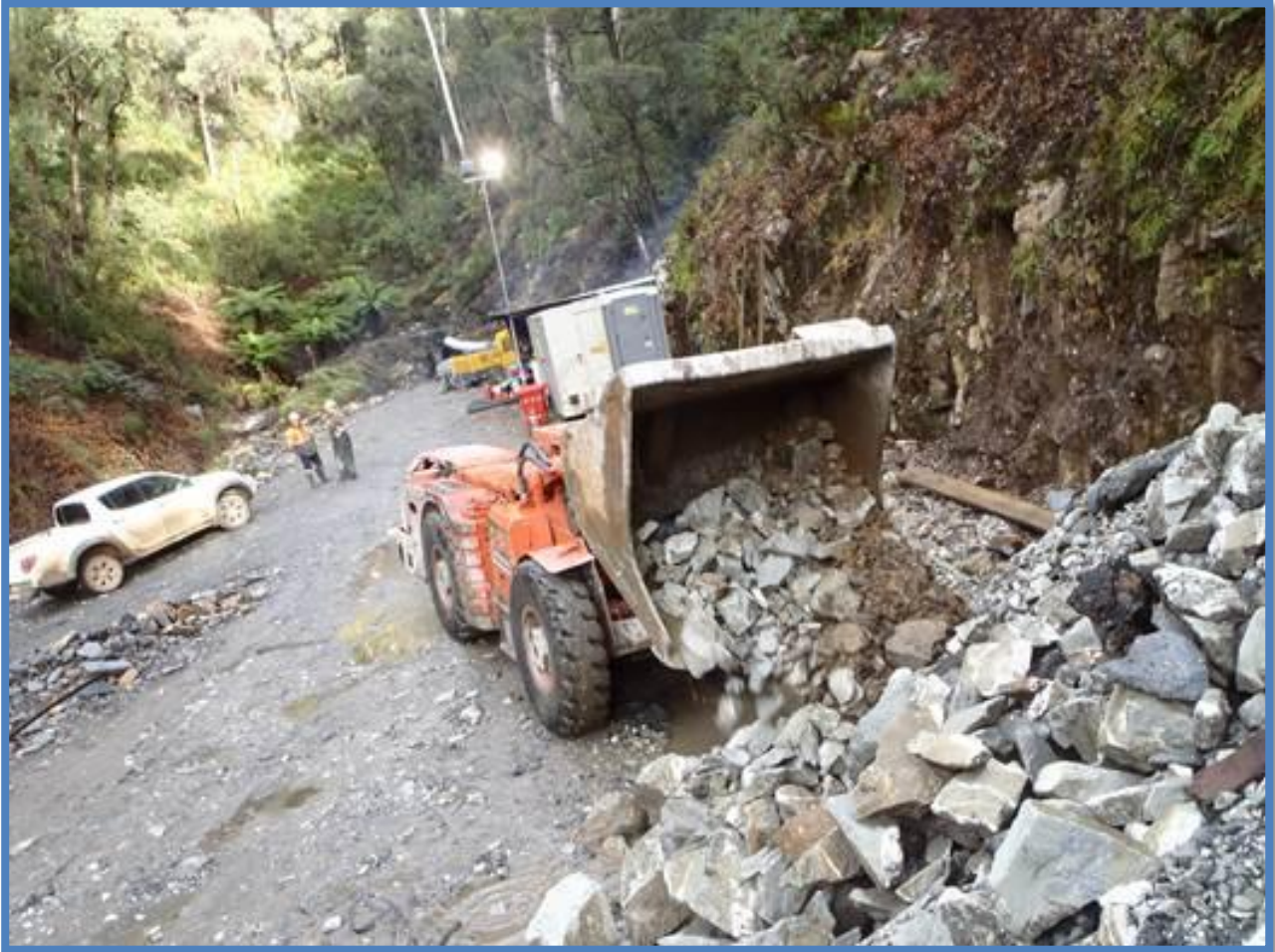
Fig 7: Mineralised Dyke from Adit being stockpiled at RoD minesite
