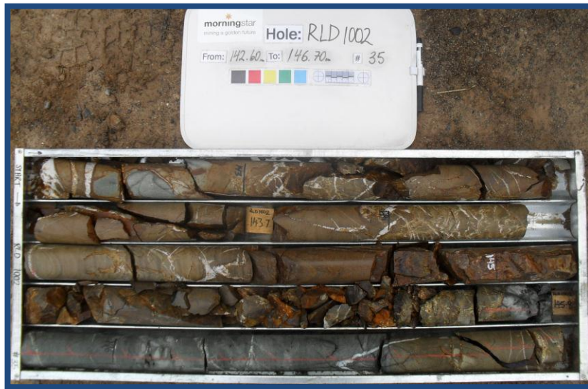
Image of Reliance Hole 2 (RLD1002) showing drill core & alteration
