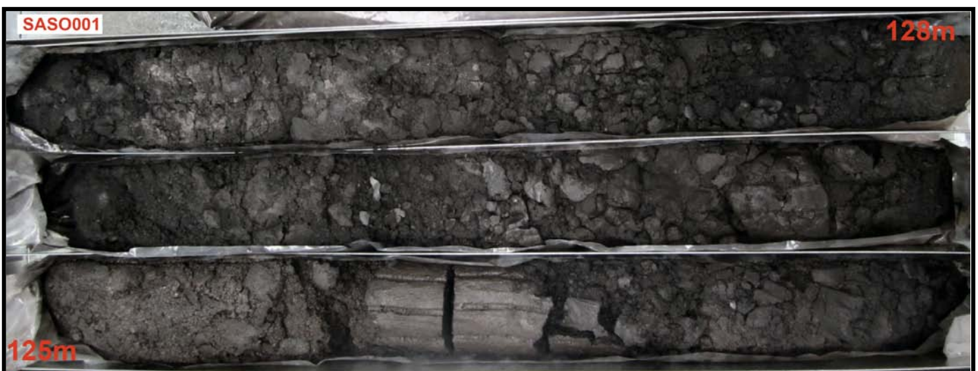
Figure 2: Example of good quality mineralised drill core sample intercept from sonic drill hole SASO001 located at Saffron . Mineralised interval within organic rich sediments.
