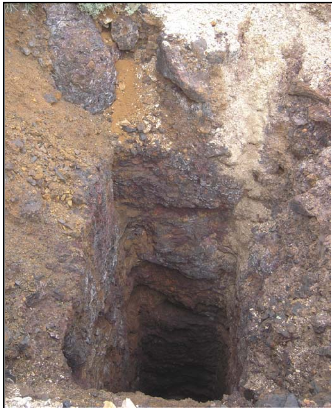
Figure 2: Photograph of historic mine shaft with visible iron mineralisation extending to depth at outcrop 4.
