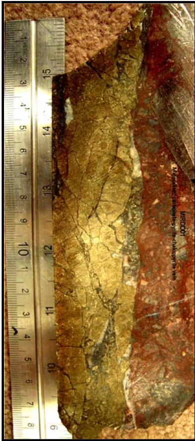
Figure 8a: Example of copper mineralisation (chalcopyrite) observed in Miranda drill hole MIRDD01 during 2010 Phase 1 drilling.
