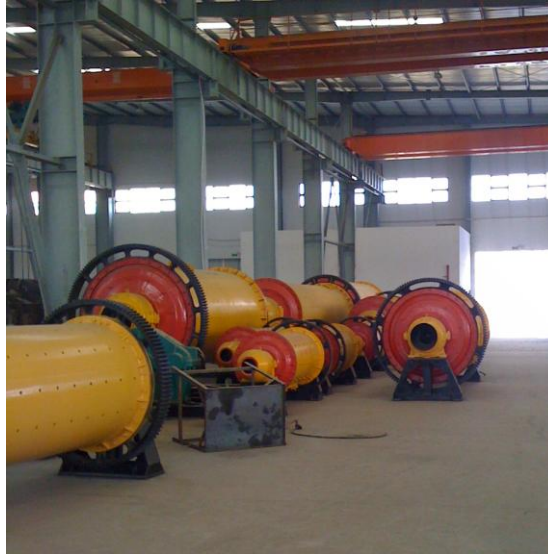
Fig 3. Examples of ball mills and driers being manufactured by one of the factories
