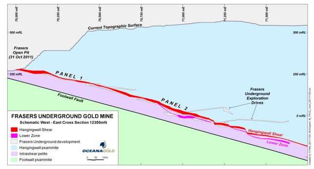
Figure 3 - East-west cross section through the Frasers Underground showing Hangingwall Shear, Lower Zone and underground development.
