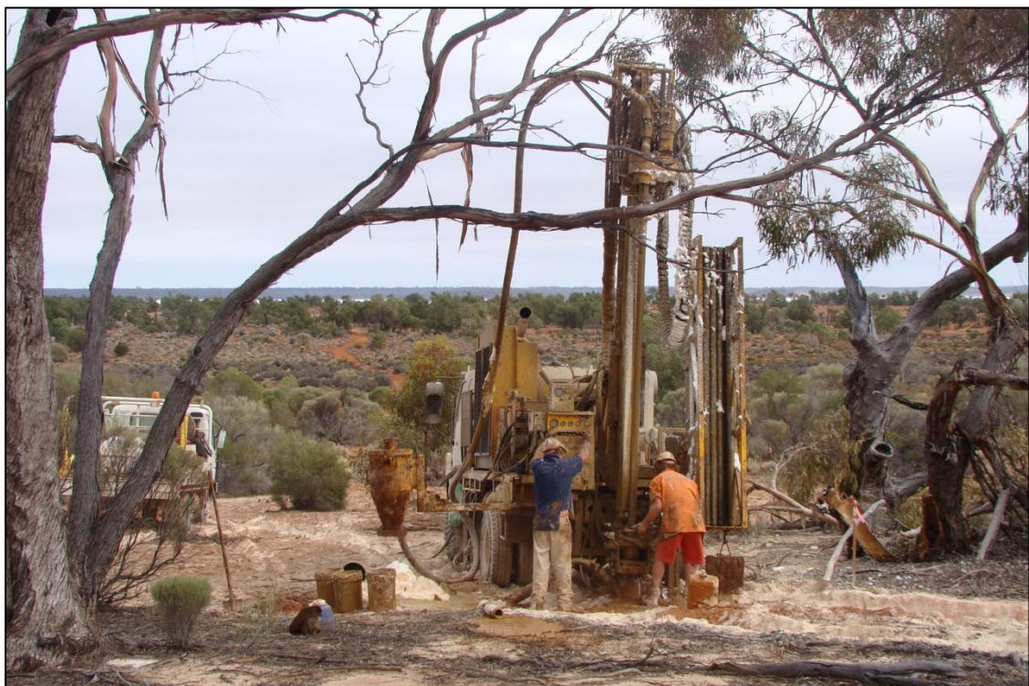
Figure 5. Burns Prospect: Aircore drilling
