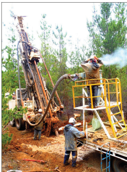
Figure 3 – Reverse Circulation Drilling at the Barnes Hill Project, Tasmania
