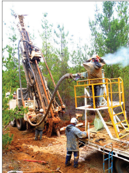
Figure 1 – Reverse Circulation Drilling at the Barnes Hill Project, Tasmania
