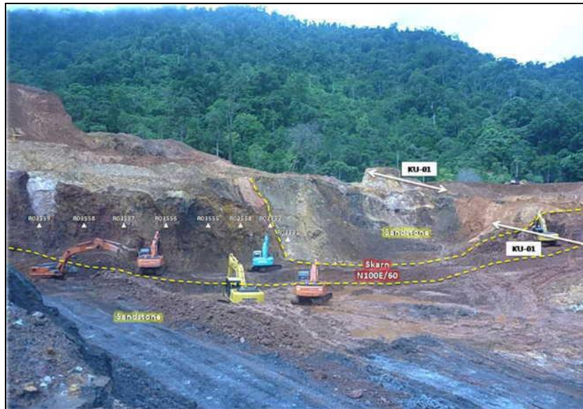
Figure 5: View of surface outcrop of Kuini skarn fully contained within Prosperity’s ATP IUP. The magnetic expression of this zone extends for some 600-650 metres along the trend of the cleared ridge line.
