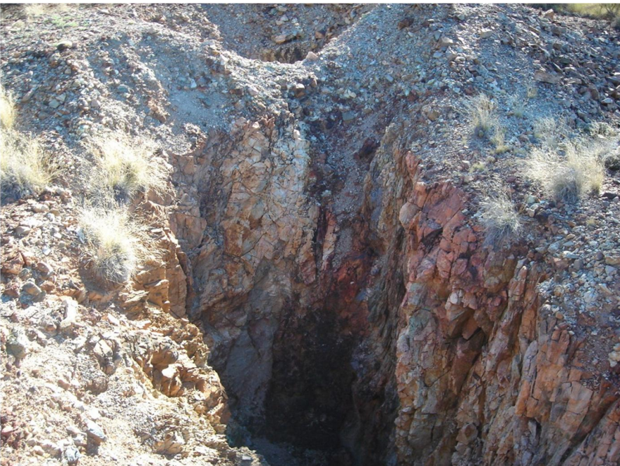
Fig. 4 'Just Luck' open pit showing exposure of the various copper minerals –including malachite and the iron oxide zone. Sulphide mineralisation in the form of chalcopyrite and pyrite veins and disseminations evident from the mullock around (looking northeast)
