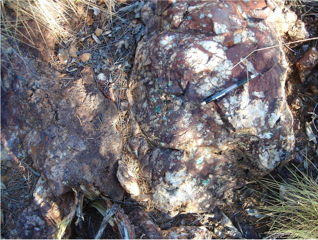
Fig. 3 Outcrop of Malachite-hematite-quartz breccia in the southern part of the Western Zone
