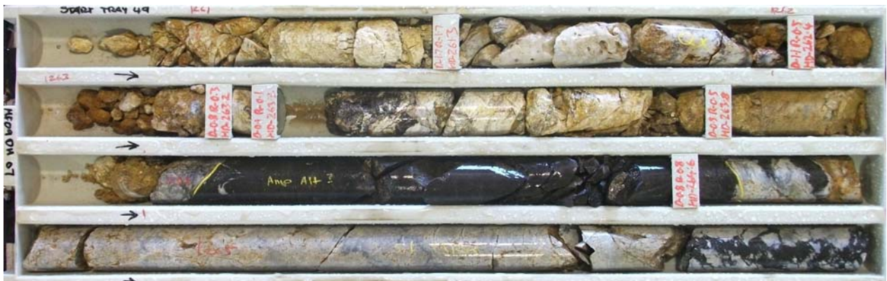
Figure 4: Core from DH07 the deepest drill hole at Mt Freda showing the weathering profile extends to a depth of more than 264m. The mineralized interval shown in the core photo (light brown colour) returned 1.65m @ 4.79 g/t Au, including 0.2m @ 9.42g/t Au from 263m (dark brown colour). Noting the substantial low recovery of core due to broken ground
