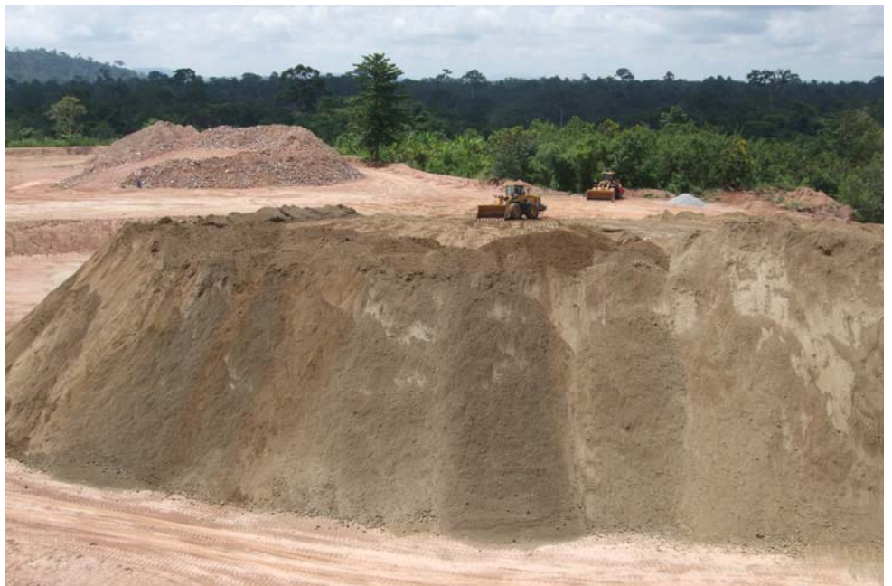
Stockpiled tailings material on the ROM pad, as seen from the plant
