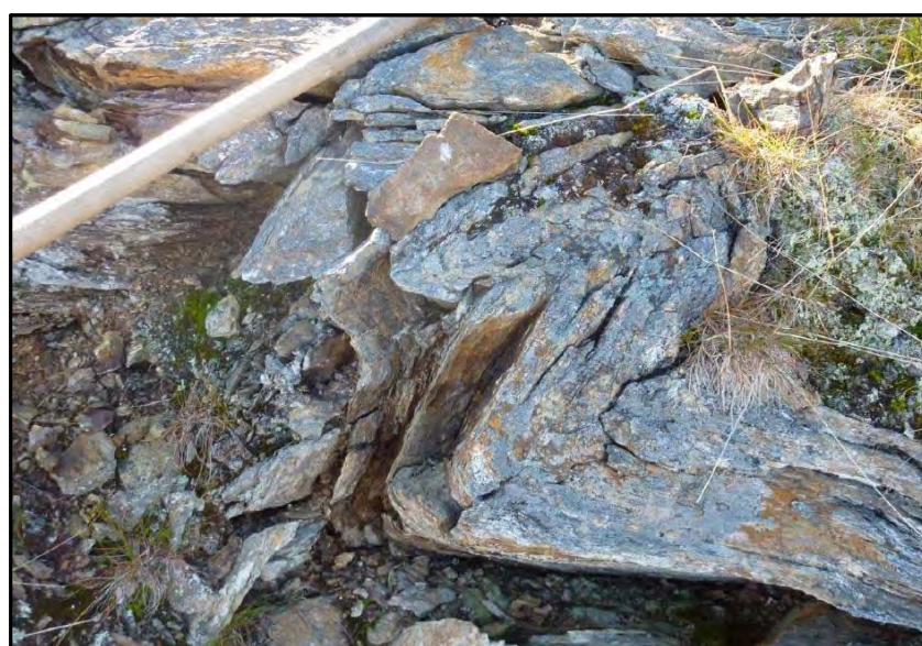
Figure 1: Intensely folded quartz sericite schist hosting high grade gold and base metal mineralisation (SAR10005 & SAR10006)
