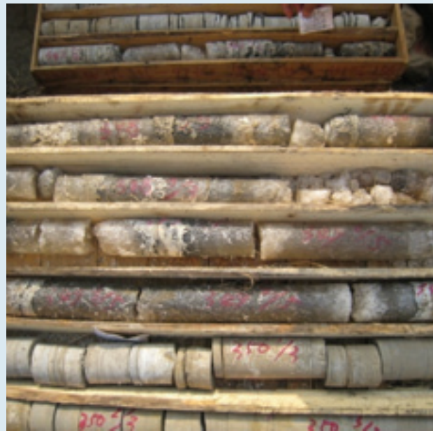
Gypsum core samples extracted from the Taian deposit in Taian, Shandong Province, China.
