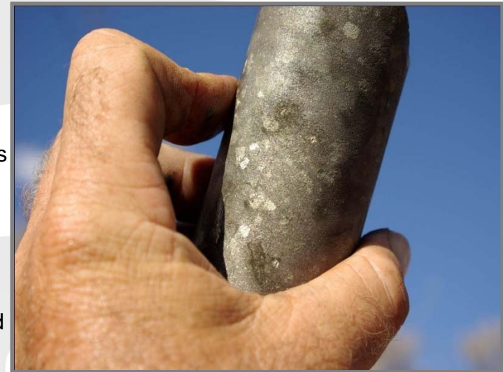
High grade nickel - copper – PGE mineralisation from the Duketon Nickel Project W.A.
