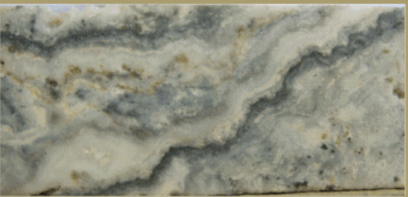
Quartz-chalcedony-adularia(?)—calcite vein with sphalerite+pyrite from Belinau (RDD10091; 4.05m @ 15.5 g/t Au from 159.1m)
